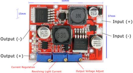
The LM2577S/LM2596 DC 4-35V to 1.25-25V automatic buck-boost converter, max output current 3A, output power 5W, automatic buck-regulator circuit, applicable high power led driver, solar panels.
