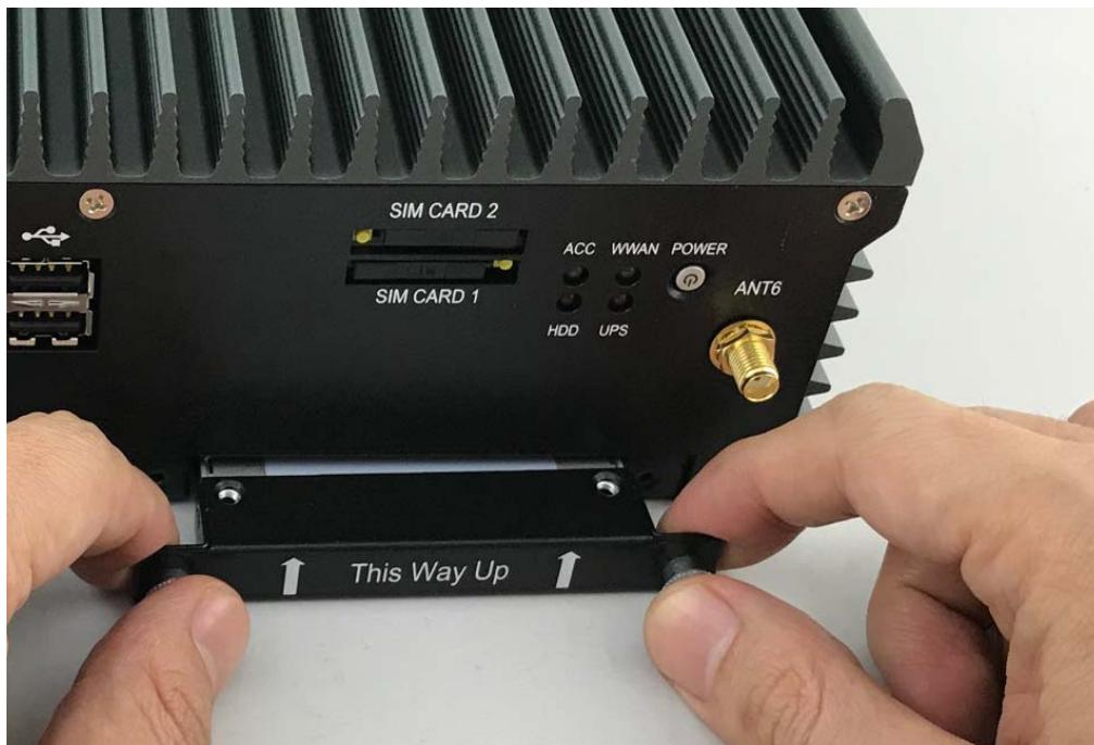
**Step 4.** Fully insert the HDD Holder into the socket until a “click” is heard as shown in the picture.
