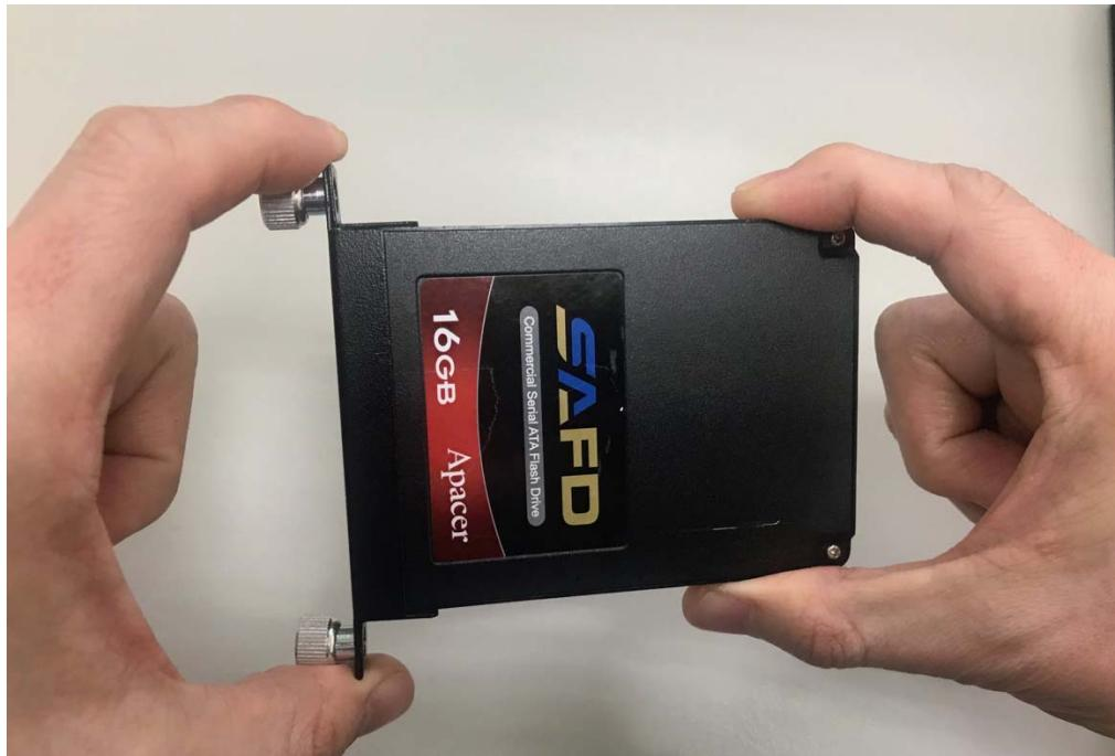
**Step 2.** Screw two screws on both side as shown in the picture.
