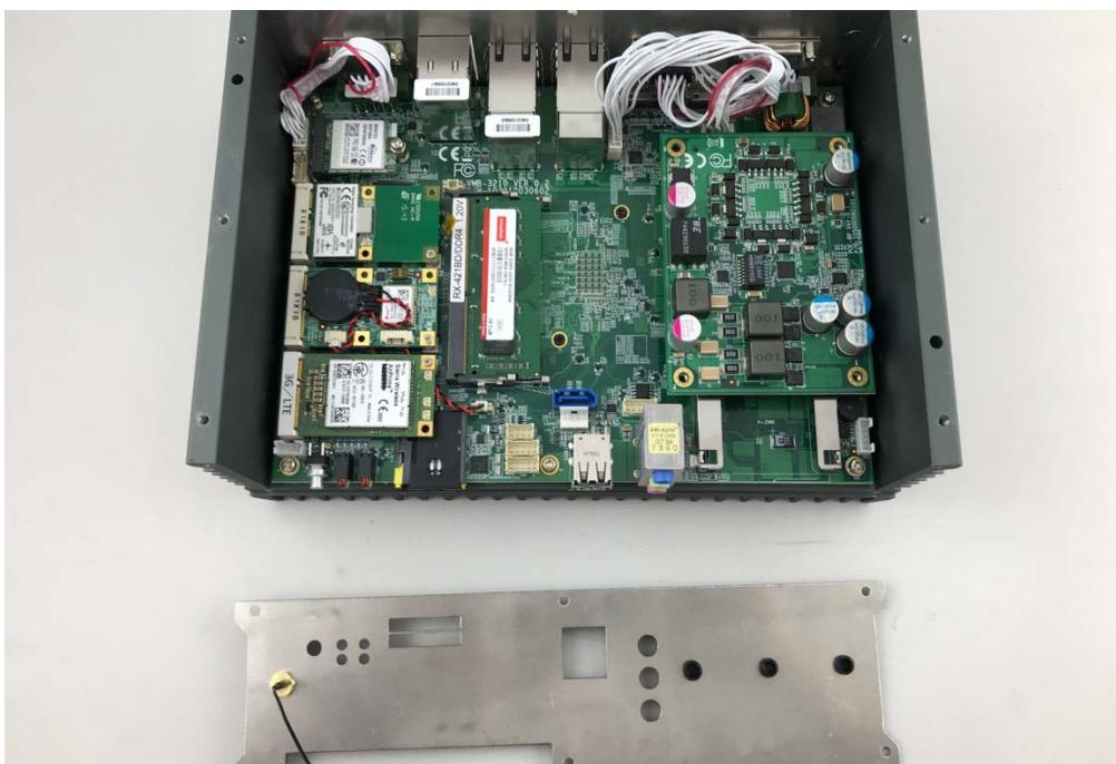
**Step 3.** Take CFast Card into the holder as shown in the picture.
