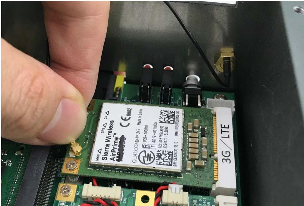
**Step 6.** Take the Ipxe Connector and press on the GPS module as shown in the picture.
