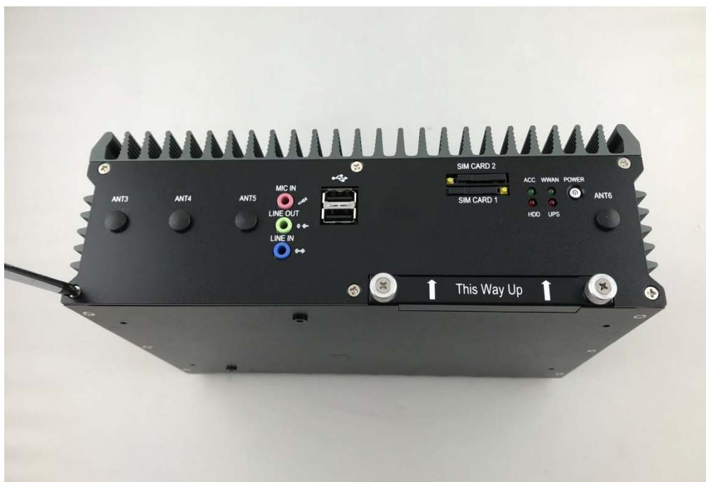
**Step3.** Unscrew the three screws of the Rear Panel as shown in the picture.
