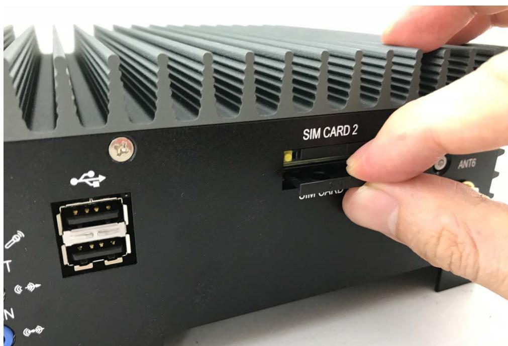
**Step 3.** Put your SIM Card into the holder and take the SIM card holder and Insert it into the socket as shown in the picture.
