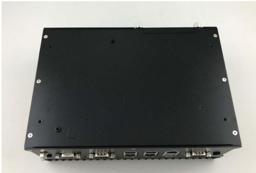
**Step2.** Unscrew the three screws of the Front Panel as shown in the picture.
