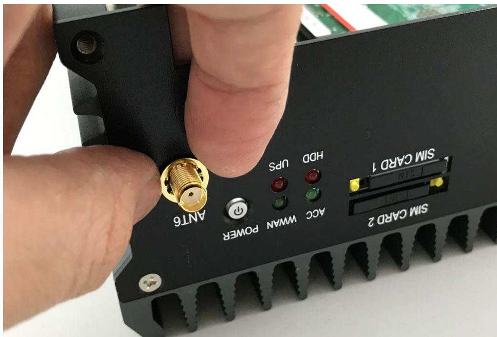
**Step 3.** Put the O-ring to SMA Connector and tighten as shown in the picture.
