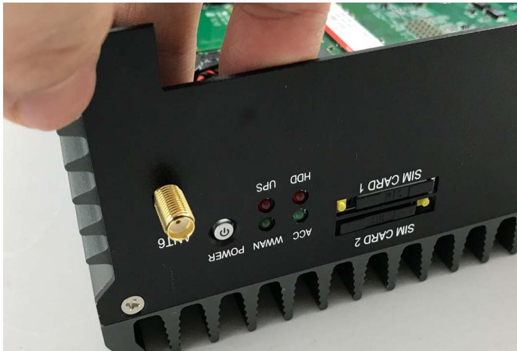
**Step 2.** Put the Washer into the SMA Connector as shown in the picture.
