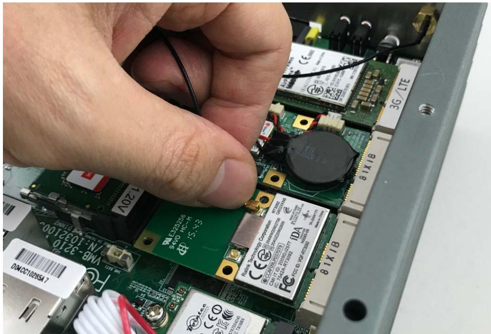
**Step 8.** Take the Ipxe Connector and press on the M.2 module as shown in the picture.
